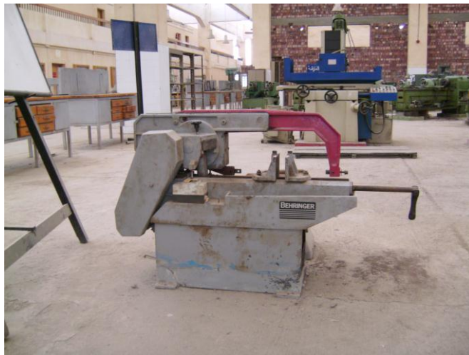
Fig. 8 Power Hacksaw Model HSH 250
